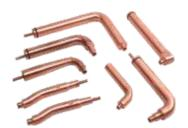
These are made of Cr Cu, Cr Zr Cu and Co Be Cu depending on the size, shape and strength requirements. Cold Bending process ensures longer life over the casting process. Copper tubes for efficient cooling are incorporated during manufacturing process.
